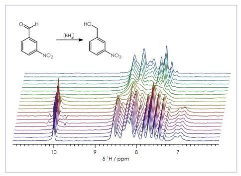
Figure 2: Time series NMR data of the reduction of 3-nitrobenzaldehyde.
